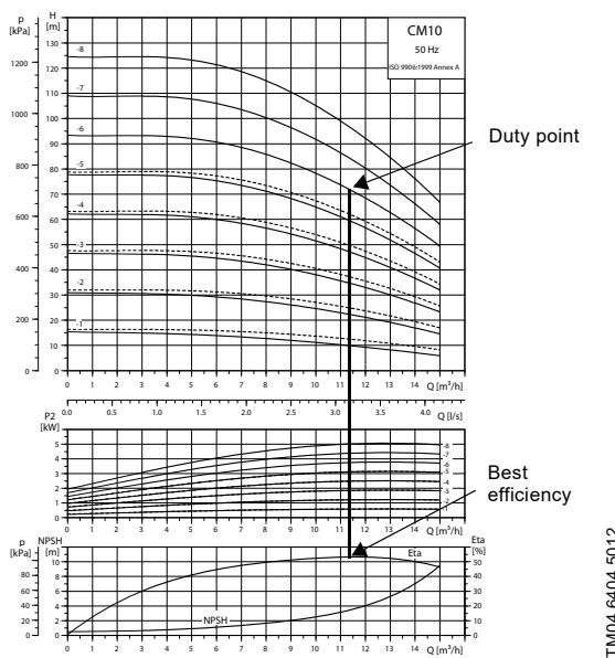
Fig. 36 Example of a CM pump's duty point
