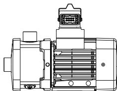
Fig. 40 Motor with a multiplug connection
