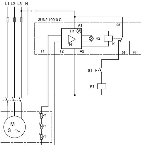
**Fig. 49** Three-phase motor with PTC sensors
