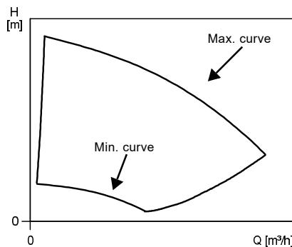
Fig. 29 Minimum and maximum performance curves
