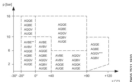
**Fig. 12** Curve for the selection of AQQx, AQBx and AVBx shaft seals
