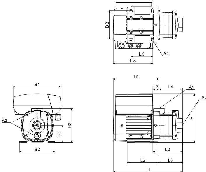
**Dimensions****3 x 380-500 V, 50/60 Hz (supply voltage S)****3 x 440-480 V, 50/60 Hz (supply voltage T)**
