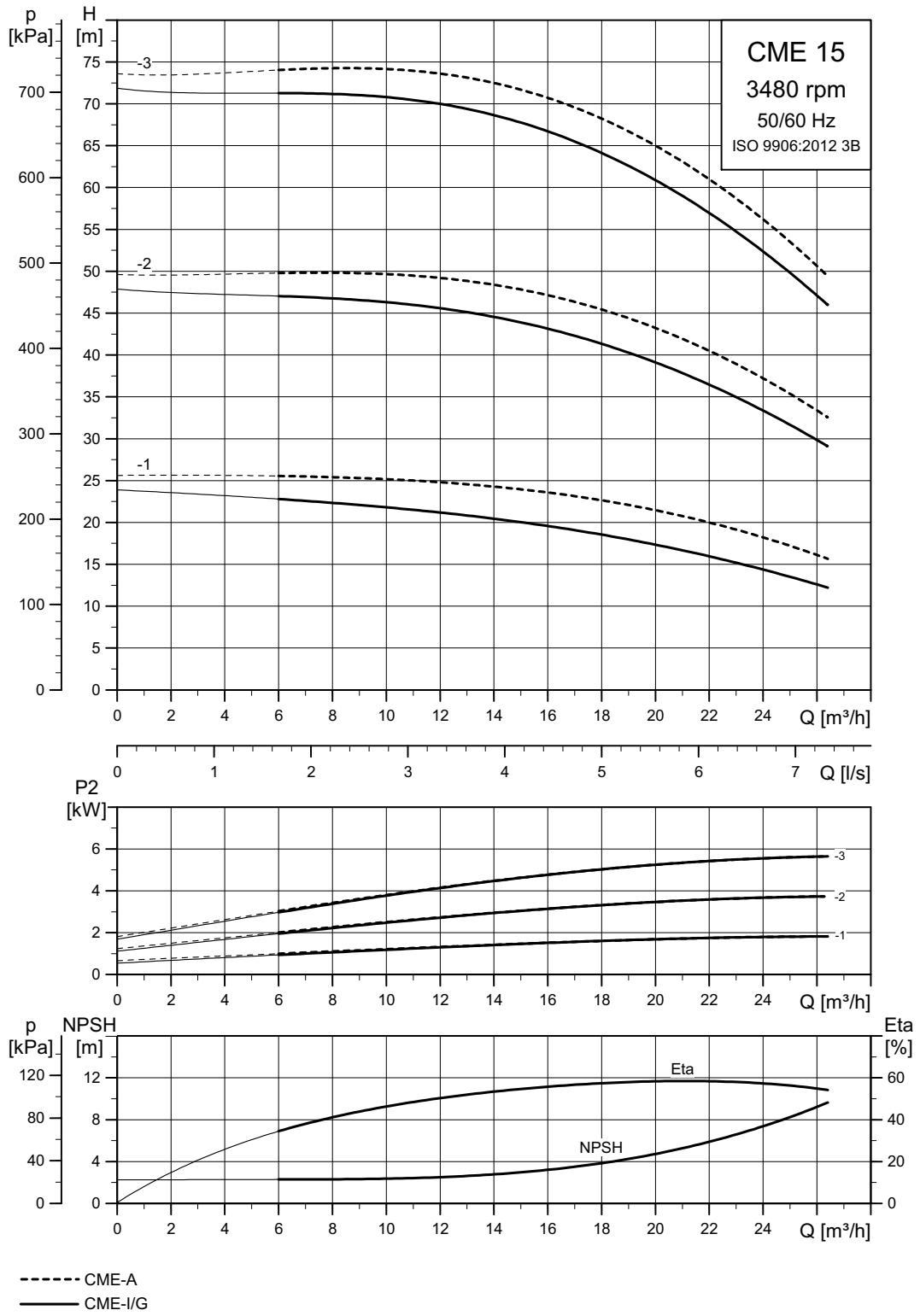
Irrespective of the input frequency, the 100 % speed of CME pumps is approximately  $3400 \text{ min}^{-1}$ .
