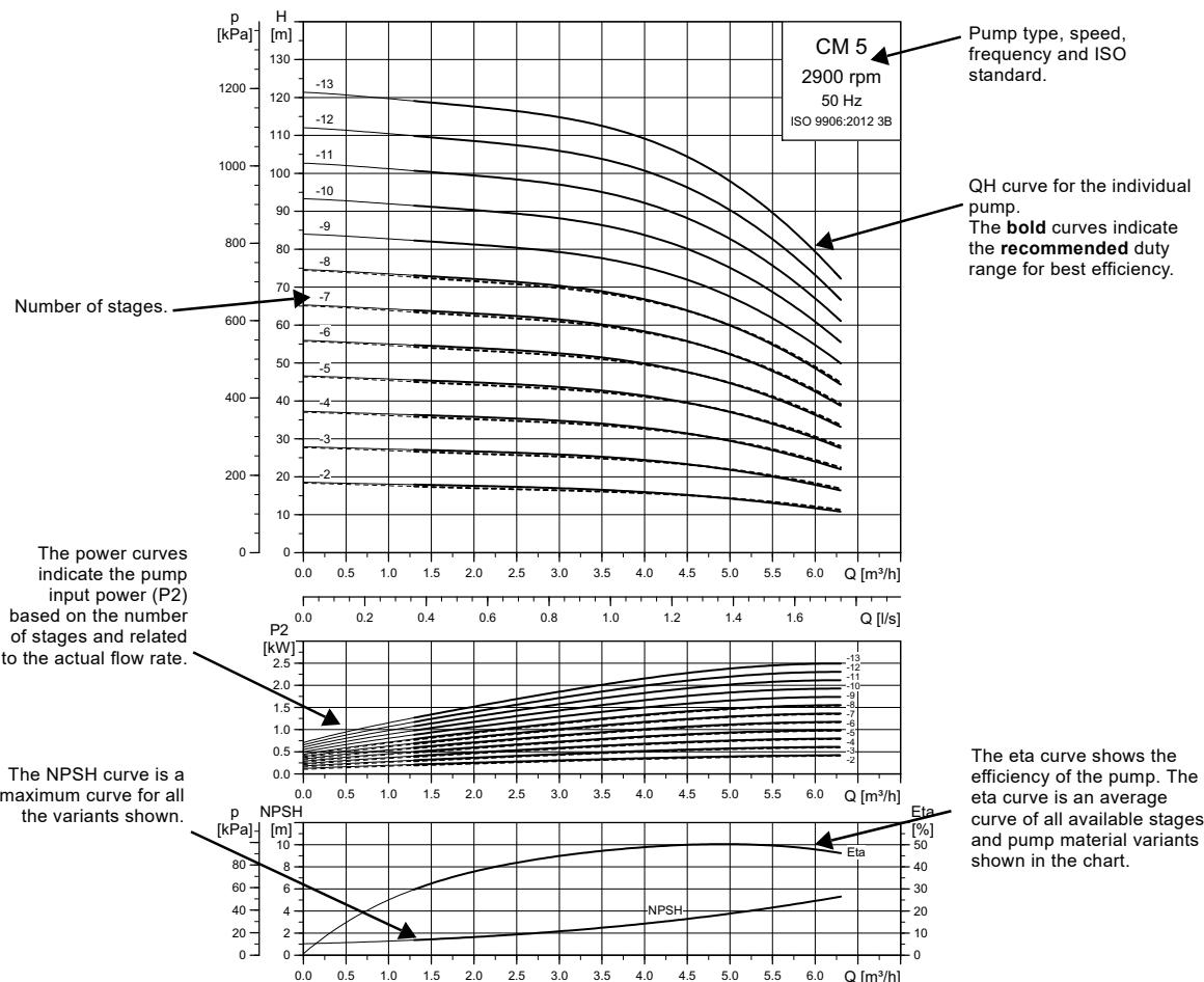
Fig. 38 How to read the curve charts
