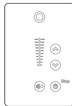
**Fig. 28** Standard operating panels of CME pumps
