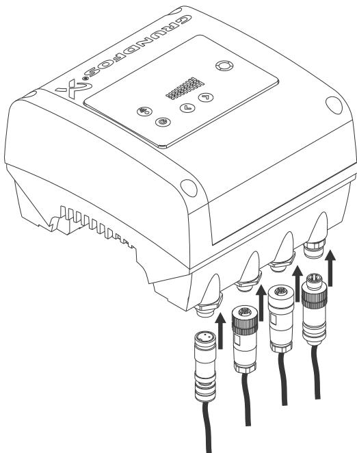
Fig. 45 Fast connection of CME pumps
