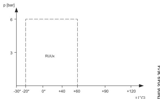
**Fig. 13** Curve for RUUx shaft seal
