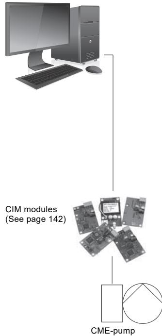
**Fig. 26** Structure of a central management system
