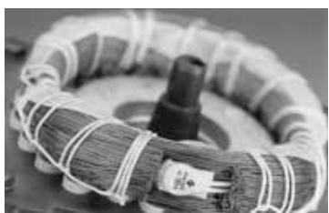
**Fig. 50** Thermal switch incorporated in windings
