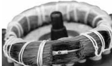
**Fig. 48** PTC sensor incorporated in windings
