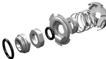
Fig. 6 Exploded view of shaft seal
